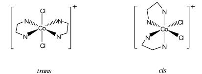
At low concentrations the green *trans*- $[Co(en)_2Cl_2]^+$  ion undergoes a first order acid hydrolysis reaction, and a red mixture of the *cis* and *trans* isomers of  $[Co(en)_2(H_2O)Cl]^{2+}$  complex ion are formed as shown below.
