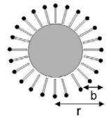
When r is the radius of the total microemulsion droplet, b the length of the surfactant molecule and r-b the radius of the polymer particle, you obtain:
