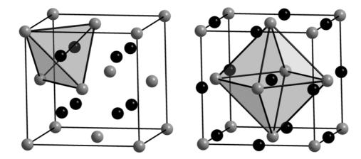
The elemental cube of a face centered cubic structure contains 4 packing atoms (one at the corner and three on the faces of the cube), eight tetrahedral holes (one in each octant of the cube) and 4 octahedral holes (one in the centre of the cube, 12 additional holes in the middle of the edges of the cube, each shared of 4 cubes).
