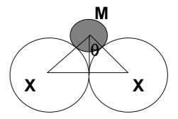
A line perpendicular to the edge divides the tetrahedral angle into two halves. The length of the edge is 2  $r_X$ . The distance from a tetrahedral vertex to the center is  $r_M + r_X$ . The angle is 109,5°/2.
