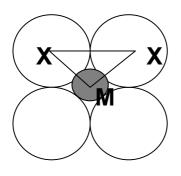
$\begin{array}{ll} (2r_x)^2 &= (r_M + r_x)^2 + (r_M + r_X)^2 \\ 4r_x^2 &= 2 \ (r_M + r_X)^2 \\ \sqrt{2} \ r_X &= r_M + r_X \\ r_M/r_X &= (\sqrt{2} \ -1) = 0.414 \\ r_M/r_X &= 0.414 \end{array}$
