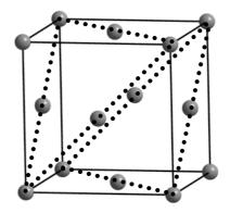
10.4 In this illustration, the atoms touch on the face diagonals. The length of the edges of the cube is  $2r \cdot \sqrt{2}$ . There are 4 complete atoms in the cube (8 corners with one eight of an atom in each and 6 sides with one half of an atom in the middle of each). So the packing efficiency is:
