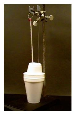
*Notes:* The inner cup can be replaced as needed, which is why there are extra foam cups. 250 mL (8 oz) foam cups may also be used but 190 mL (6 oz) cups are not recommended. You may choose to supply a ring clamp to stabilize the base of the cup assembly. Another option is to place the cup assembly in an appropriately sized beaker that serves to support the cups and to provide extra insulation.
