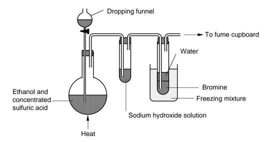
The mixture in the flask was heated to about 170°C. Ethene (ethylene) was formed and reacted with the bromine in the second test tube to form 1,2-dibromoethane.
