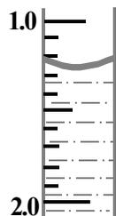
The above diagram shows the cross section of a burette that is partially filled with a solution. What is the burette reading?
