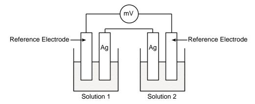
Two silver electrodes, connected by a copper wire, are immersed in two initially identical solutions, prepared by mixing 50 mL of 0.010 M  $AgNO_3$  solution with 50 mL of 0.10 M  $NH_4NO_3$  solution. Two identical reference electrodes are also immersed in the solutions and are connected through a millivoltmeter.
